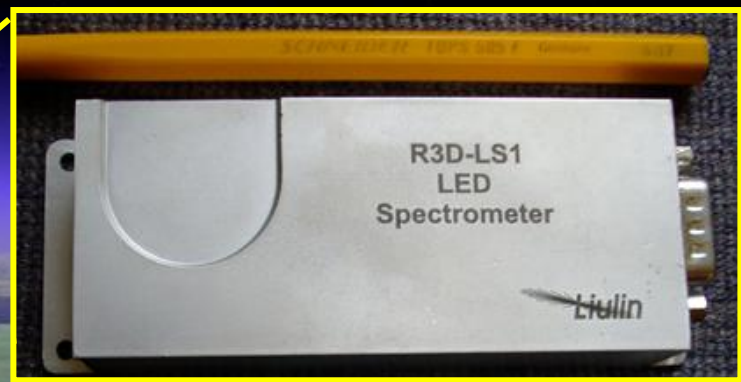
Expected appearance of "Liulin-AF" spectrometers
