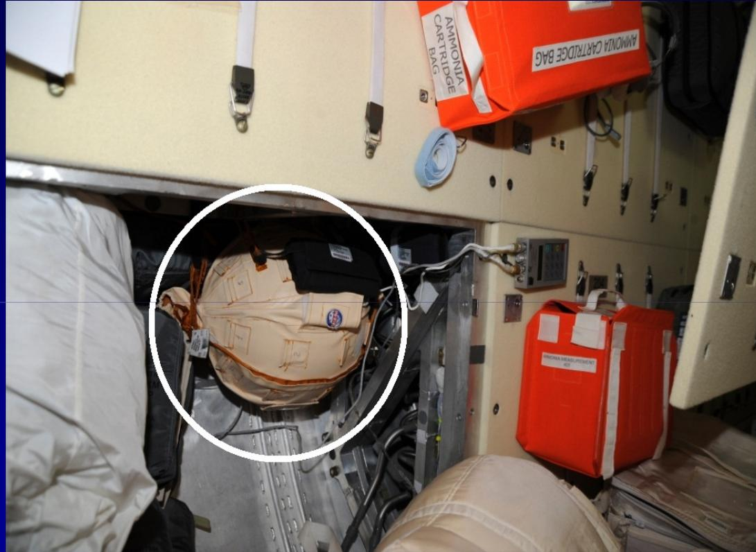
The spherical phantom on ISS, located in the MRM1 module behind the panel 206. Inside the phantom (behind the label) is the detector module of Liulin-5.
