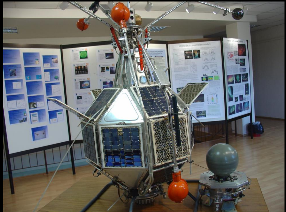
Engineering model of the satellite MAGION 2 exhibited during Open door days at Institute of Atmospheric Physics
