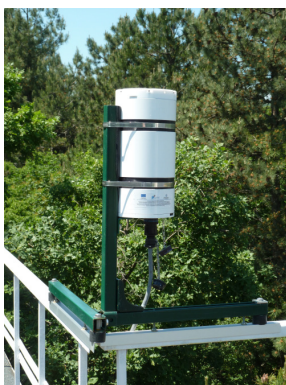
Fig.2. View of the GUV 2511 instrument on the roof of the observatory.
