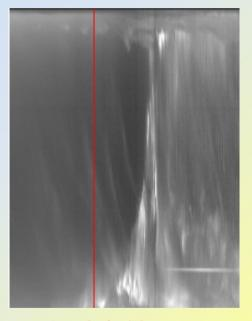
17:36:40 AS keogram 17:23-18:00 UT The substorm development can be followed by the AS images and keograms. The substorm was seen from Apatity in 17:36:40 UT on 17.03.2015 to the South of the station. In 17:42 UT a fast motion towards North was observed and in 17:45:30 UT the auroras occupied the whole field of view.
