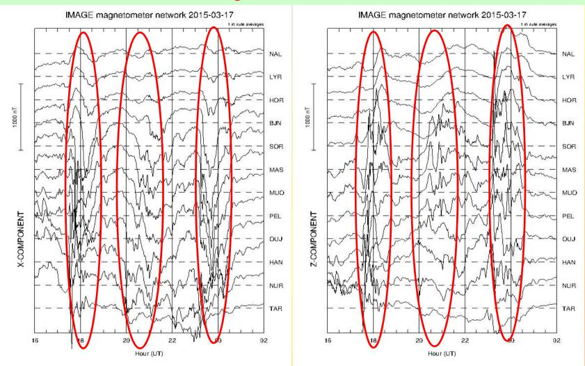
Magnetic field data, 17.03.2015. The substorm times are marked by red ellipses.
