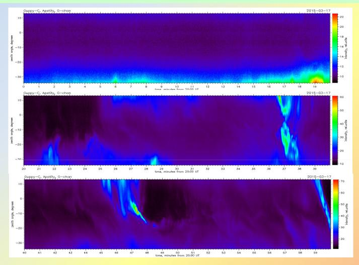
The substorm by the GC keogram from 20:00 to 21:00 UT. The auroras are seen at about  $25^{\circ}$  to the South from zenith (the upper picture) and the rise in 20:24:30 UT is clearly expressed.
