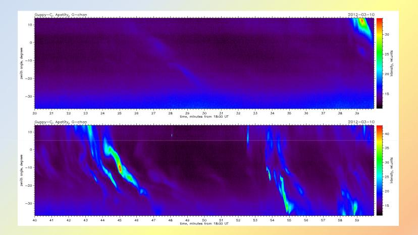
The substorm by the GC keograms from 18:20 to 19:00 UT. In the keograms, the substorm auroras are seen from 18:38:30 UT at about 15° to North from zenith.
