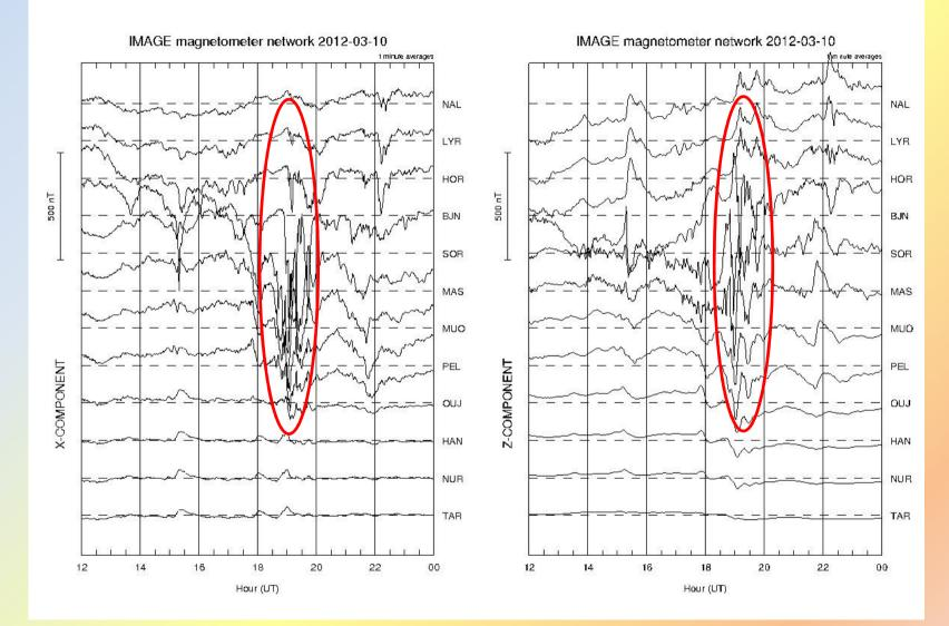
Magnetic field data, 10.03.2012. The substorm time is marked by a red ellipse.
