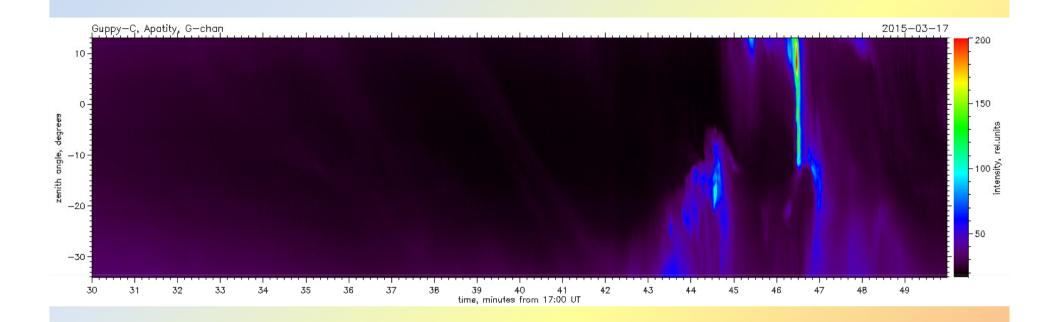
The substorm by the GC keogram from 17:30 to 17:50 UT. In the keogram, the substorm auroras are seen from 17:42:30 UT at the South part of the field of view, at 35° from zenith, due to the fast movement to North.
