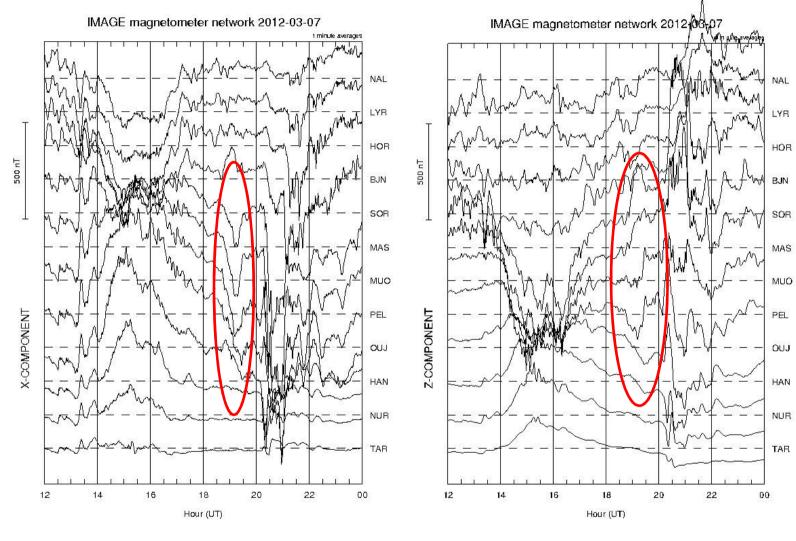
Magnetic field data, 7.03.2012. The substorm time is marked by a red ellipse.
