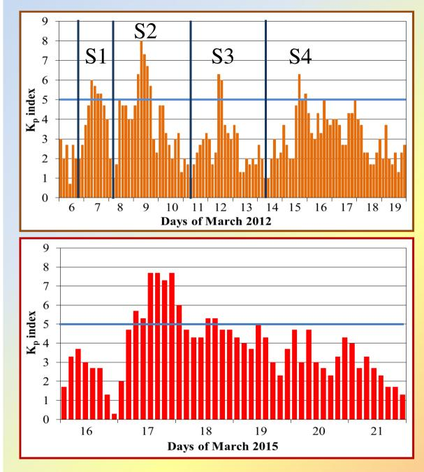
k<sub>p</sub> index variations during the examined periods. The border of the "storm" conditions is marked by the blue vertical line. During the first period there are 4, relatively short, periods of storm activity, named events S1, S2, S3 and S4. During S2 the level of severe storm was reached, the others are at the level of moderate storms. In the second period, a fast increase of k<sub>p</sub> was observed, and it reached the level of severe storm.
