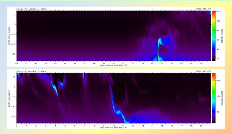
The substorm development by the GC camera keograms 18:40 - 19:00 UT and 19:00 - 19:20 UT. In the GC keograms the substorm auroras are seen first in 18:52 UT. The substorm development is clearly expressed up to 19:20 UT.
