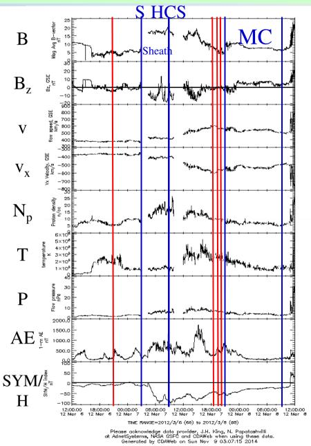
Interplanetary conditions during 6-8.03.2012 and substorm times Interval 1: 6-8.03.2012: Halo CME, MC1 Sheath: from 03:28UT, 7.03.2012 MC: 21:30 UT, 7.03.2012 to 9:20 UT, 8.03.2012 Geomagnetic storm: min Dst = -98 nT
