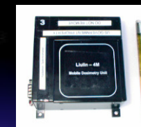
Liulin-MD Liulin-MDU-5 type flown for more than 6000 hours on CSA aircraft
